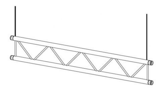
H40L has thicker diagonals than H30L and can take slightly heavier loading
