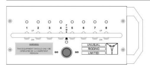
The standard hand held unit is designed to give full up /down control over 8 or 16 hoists at one time. The remote consists of 3 position switches with adjacent LEDs to give an indication of the direction the hoist will travel when the go button is pressed. The go button is fitted centrally below the selector switches and an extra LED gives a control voltage present indication. The 16 way is similar to the eight way remote shown above, but has two rows of switches and LEDs.
