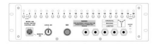
The 20 way controller is a 19" rack mounting enclosure of similar construction to the 4 way module. The front panel is fitted with 20 direction selector switches, each with adjacent LEDs, and a master Go button. A key switch selector and 3 pin xlr socket allow a remote Go button to be used. The controller is connected to the distro modules using five flying leads fitted to the front panel, one for each module.
